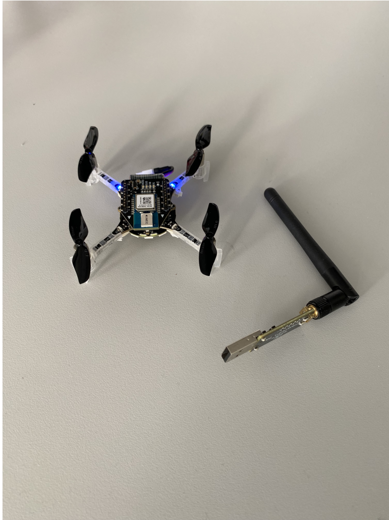
Figure 4.3: The Drone used in this project is the Crazyflie 2.1, as shown here, but the earlier version 2.0 works just as well
