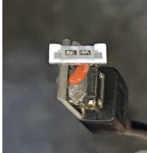
(b) Charger with straight pins (after fixing)
