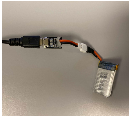
(a) Crazyflie battery charging: with micro-USB cable
