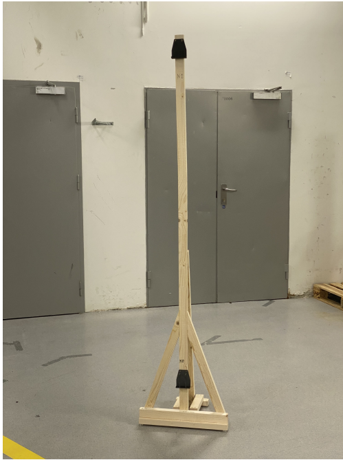
(a) The node stand which erects node holders to correct height
